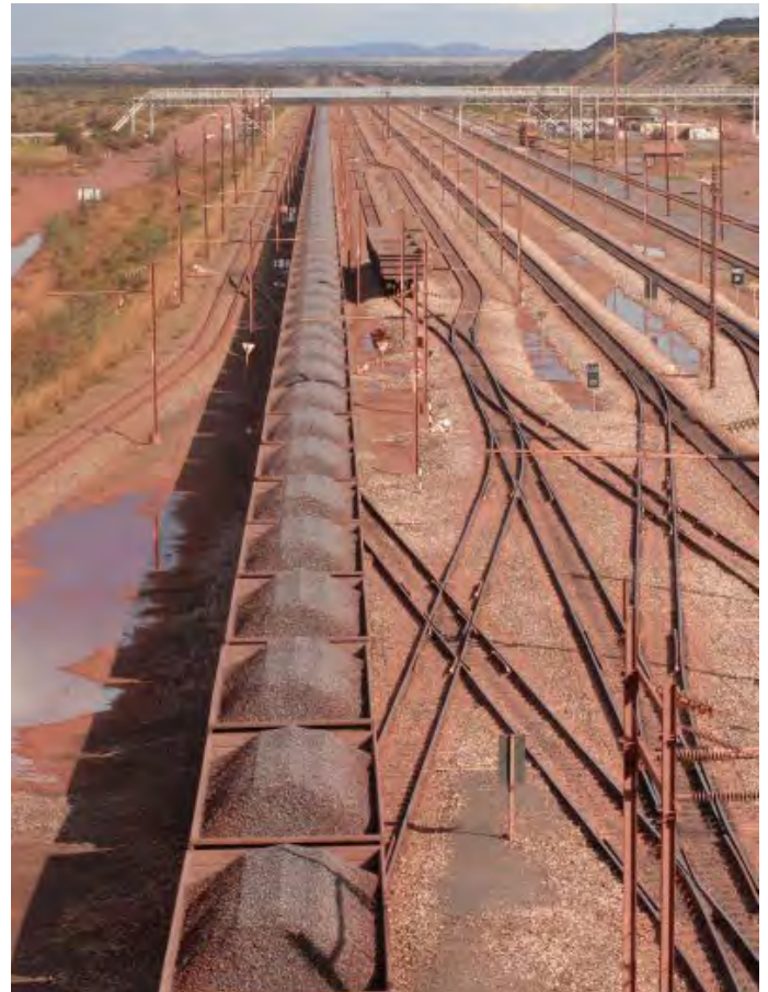
Sishen Mine, a Kumba Iron Ore mine. The loading of the Sishen to Saldanha ore train; 216 wagons of 100 tons each make up each train, Northern Cape province, South Africa. Source: Graeme Williams, Medi-aClubSouthAfrica.com
